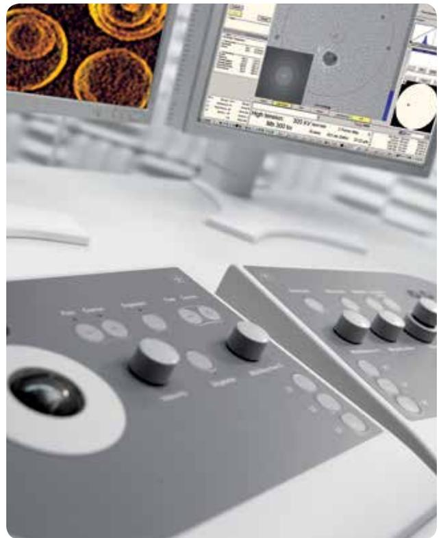
↑ Primary control unit of the Titan Krios can be placed up to 15 meters from the microscope for ease of operation.
