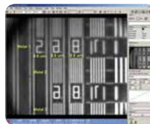
↑ View of circuitry through the backside silicon using integrated IR microscope showing resolution <0.5 \mu\text{m} .
