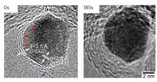
↑ Surface-step as growth centers for graphene on a Pt / MgO alkane dehydrogenation catalyst - dynamic *in-situ* ETEM study (1.3 mbar C4H8, 475°C) with atomic-scale resolution. Z. Peng, et al., J. Catal. 286 (2012) 22; Courtesy of A. Bell (UC Berkeley), C. Kisielowski (LBNL) & S. Helveg (HTAS).
