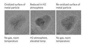
↑ Atomic resolution images of an oxidized metal nanoparticle undergoing reduction in hydrogen gas followed by subsequent re-oxidation. Courtesy of T. Hansen & J. Wagner, DTU Cen, and J. Nielsen. DTU Cinf.
