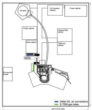
↑ Schematic drawing of Titan ETEM room layout. In addition to standard TEM room requirements (room survey, etc.), please consider space, installation, and safety requirements for gas supply, gas storage, gas inlet/mixing units and gas exhausts. Please contact your FEI representative.
