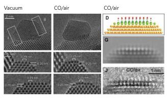
↑ Dynamic ETEM study (1 vol% CO in air gas mixture at 0.45mbar at room temperature) of carbon monoxide oxidation on Au/CeO2. Visualizing of surface reconstruction and CO gas molecules interaction with surface of Au nanocatalysts at reaction conditions. H. Yoshida, et al., Science 335 (2012) 317; Courtesy of S. Takeda (Osaka University).
