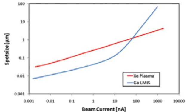
↑ Plasma FIB beam size progression continues from where the Ga LMIS beam size blows up due to spherical aberration effects.
