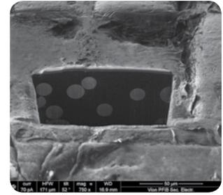
↑ After stress testing the reinforced polymer tensile test bar was sectioned and imaged by the Vion PFIB. One can observe the location and orientation of the fibers in the polymer matrix. Section width 120  $\mu\text{m}$ .
