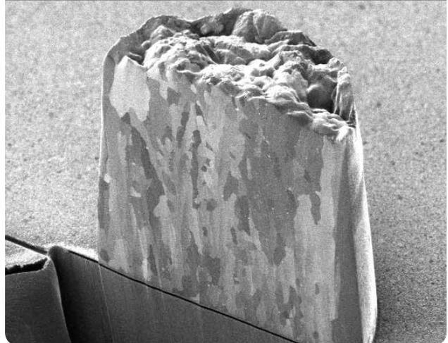
↑ An 80  $\mu$ m wide and 100  $\mu$ m tall bump cross-sectioned and imaged with Vion FIB in 20 minutes. Courtesy of SEMATECH.
